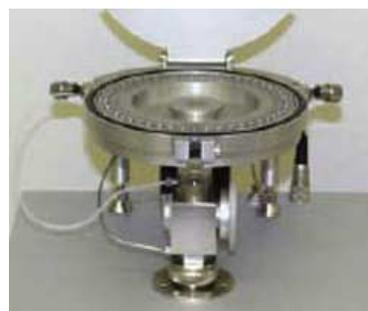
The elemental analyzer is fitted with the SmartEA option which, in conjunction with the ConFlo IV, allows the automatic dilution of the sample gas as to adjust them to the reference gas level, for each element. The range of sample weight is rather wide thanks to the automatic dilution, but a minimum of 10 µg of C and N is needed to achieve the required precision.
